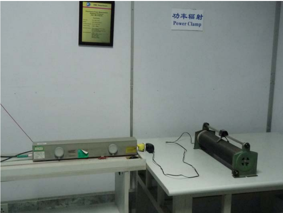
6.2.Set-up for disturbance power test
