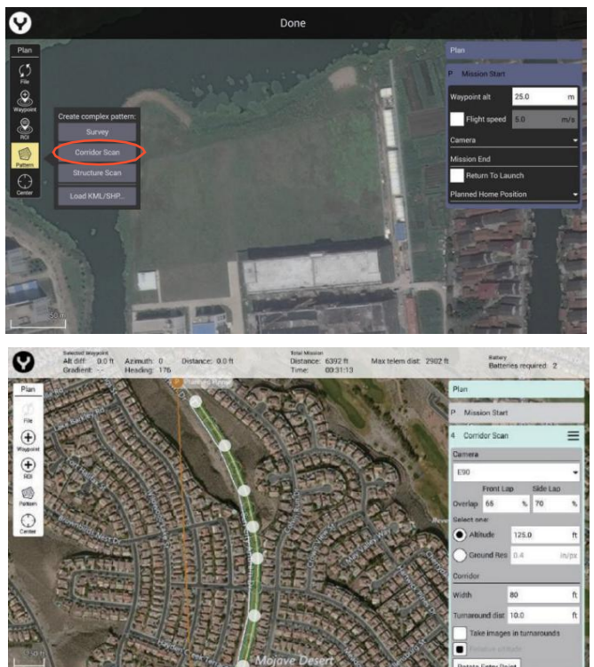
In this image, seven vertices have been inserted, allowing the Drone to follow the curvature of the roadway.
